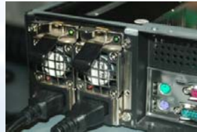
Redundant Power Supply
