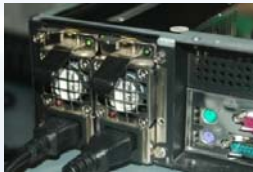
Redundant power supply Rackmount solution
